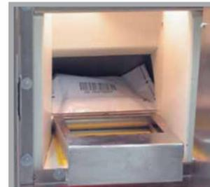
A second verification point, embedded in the structures of the drop mechanism, closely photographs the security money bag as it is being placed in the drop slot. This can be used to ensure that the security money bag has been dropped into the night deposit.
